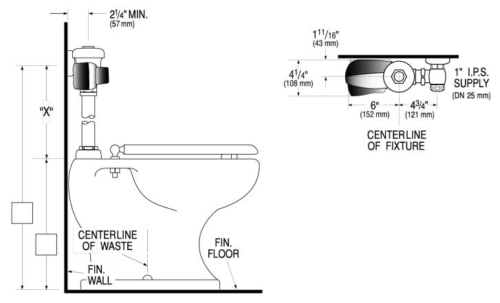
"X" = Model 113 — 16" (406 mm) Model 114 — 34<sup>3</sup>/8" (873 mm) Model 115 — 24" (610 mm) Model 116 — 27" (686 mm)
